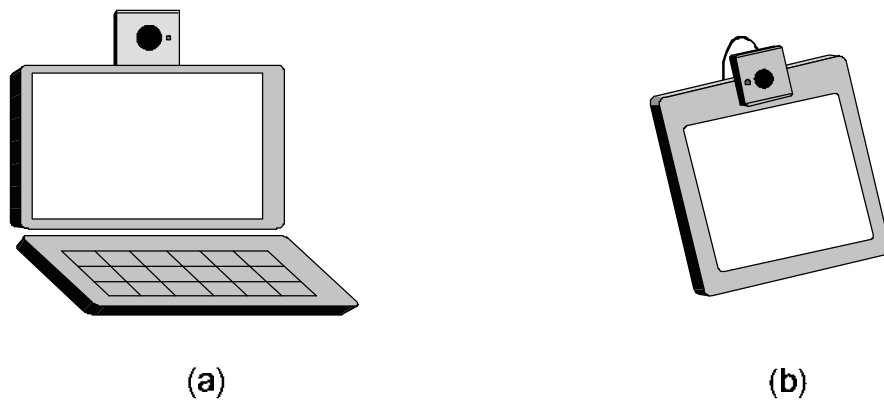
Figure 8. HeadMouse for Portables attached (a) to a laptop computer using the standard Sensor and (b) to an AAC device using the miniature Sensor. In both cases, the Sensor is attached using Dual-Lock or double stick tape.
