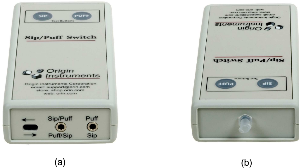
Figure 2: (a) Sip/Puff Switch electrical connectors and connector sense switch. Stereo cable should be plugged into the center connector. (b) Pneumatic connector.
