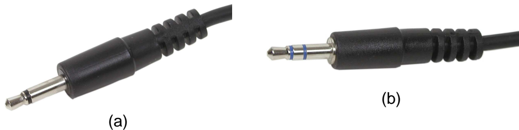
Figure 2: Mating plugs for Switchbox jacks, 1/8" microphone (3.5mm). (a) Mono plug has switched contact on the tip with the common contact on the sleeve. (b) Stereo plug has switched contacts on tip and ring with the common contact on the sleeve. Stereo cable is ALWAYS plugged into the center connector.
