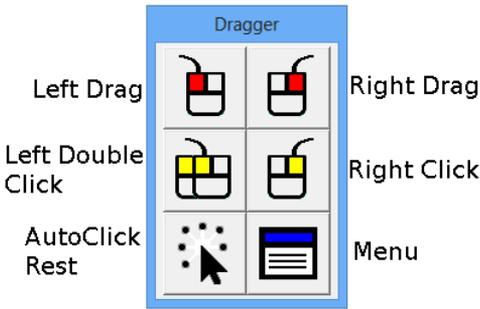
Standalone Dragger is an on-screen mouse utility that provides an alternative way for performing mouse clicks and drag operations. Dragger can be used to enter right and middle mouse clicks via direct selection (often with an adaptive switch), and by holding the mouse pointer
