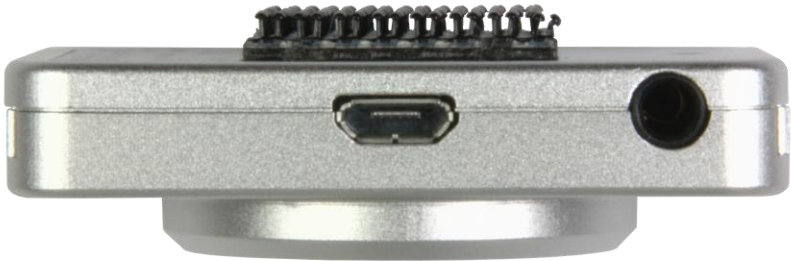
Figure 2: HeadMouse Nano Top View. USB Micro-B in the middle, and 3.5-mm jack for one or two adaptive switches.
