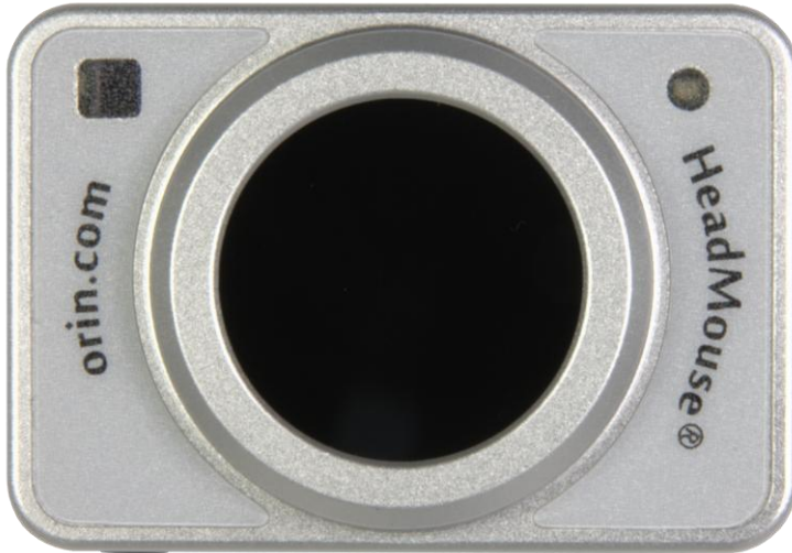
Figure 1: HeadMouse Nano Front Panel. Optical tracking sensor in the middle, infrared receiver for available Beam on the left and status LED on the right.
