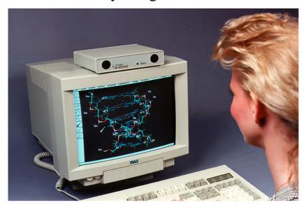
The DynaSight is a compact, self-contained sensor that measures the instantaneous three dimensional position of a passive target. The sensor uses embedded signal processing to automatically acquire and track the target in uncontrolled environments.
